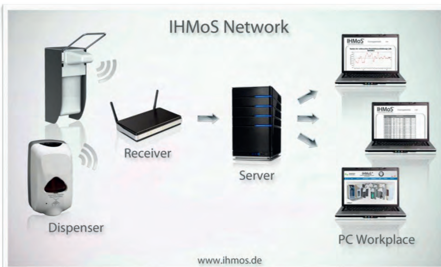
IHMoS network structure with dispensers, IHMoS receiver, server and workplace PCs
