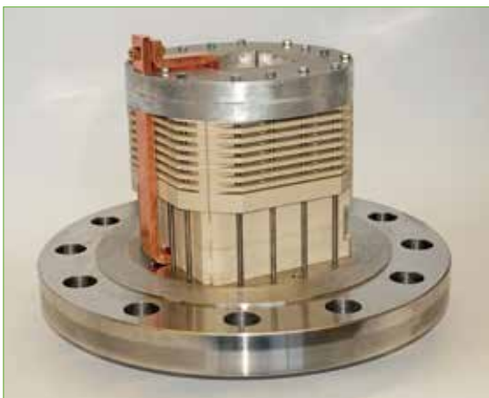
Fig. 1: Photograph of a high-pressure PEMEL stack operating on the principle of hydraulic single-cell compression.
