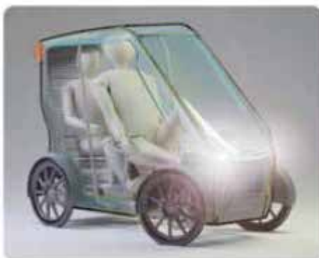
Fig.1: Concept for a two-track, roofed mobility solution, based on the pedelec and designed for use on high-speed cycle tracks (RS1 Mobil)
