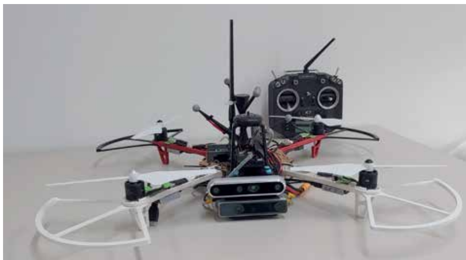
Fig. 1: General configuration of the demonstrator system: the companion computer for onboard localisation and interfacing with the additionally integrated sensors. Flight controller for direct motor control, positioning and location regulation through the use of internal sensors.
